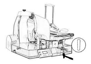
Insert the flywheel so that the manoeuvring handle is at the top and to the left, as shown in the figure, compared to the hole for the taper pin.
