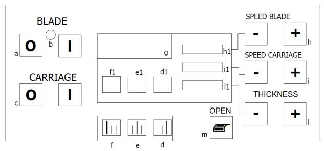
Check that the slicer is properly connected to the electrical line. The off button light (b) must be on.
